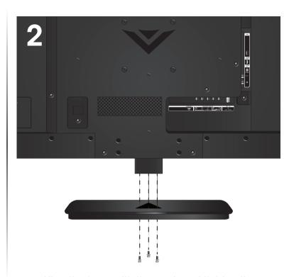
Align the base with the neck and tighten the three (3) included M4 10mm Phillips screws using a Phillips screwdriver as shown.
